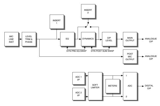
(In this example both ADC I and ADC 2 switches are lit and Soft Limiter is switched in.)
